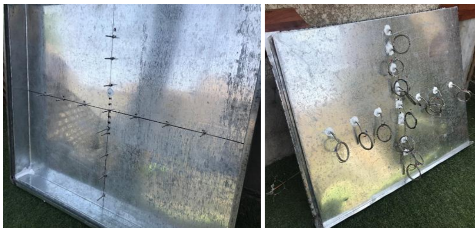
Figure 3.14: How to put thermocouples.
