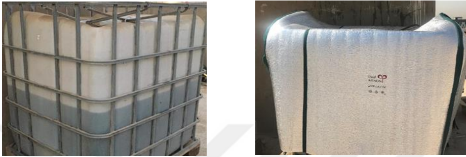
Figure 3.8: Water storage tank.
