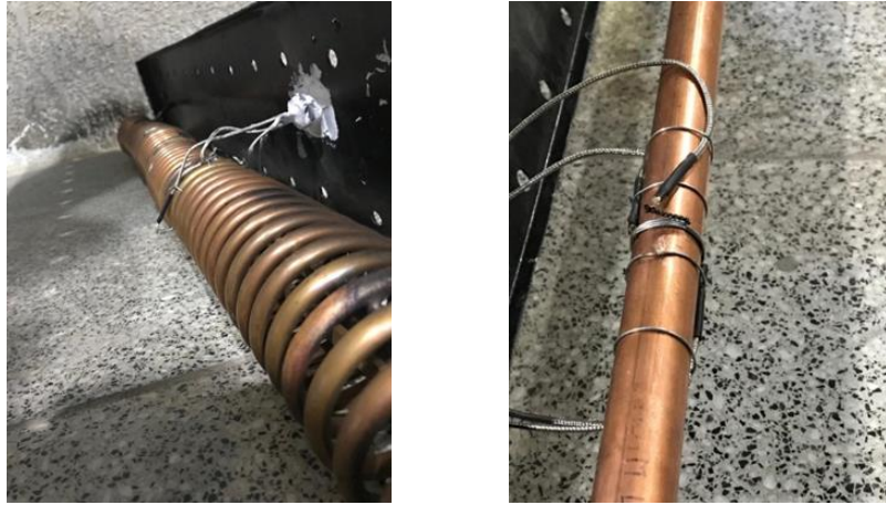
Figure 3.16: Water temperatures surrounding the tube heat exchanger.
