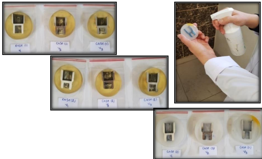
Figure 5.19: Sample polishing steps: (a) 6 \mu\text{m} , (b) 3 \mu\text{m} , (c) 1 \mu\text{m} , and (d) 0.25 \mu\text{m}
