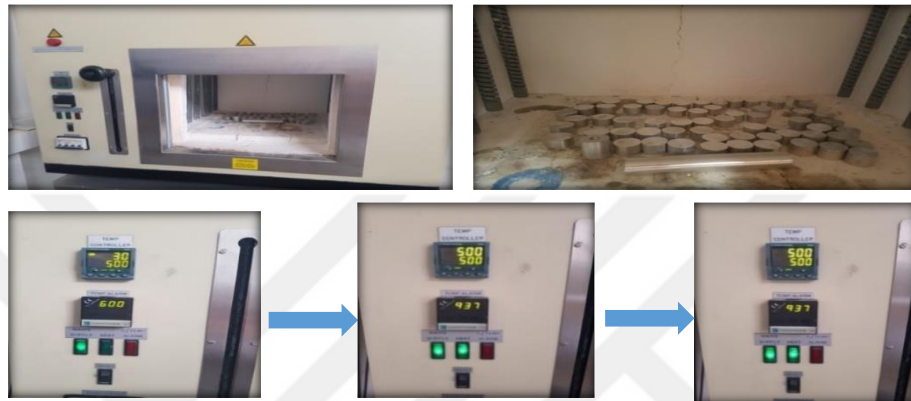
Figure 5.3: Annealing heat treatment for billets
