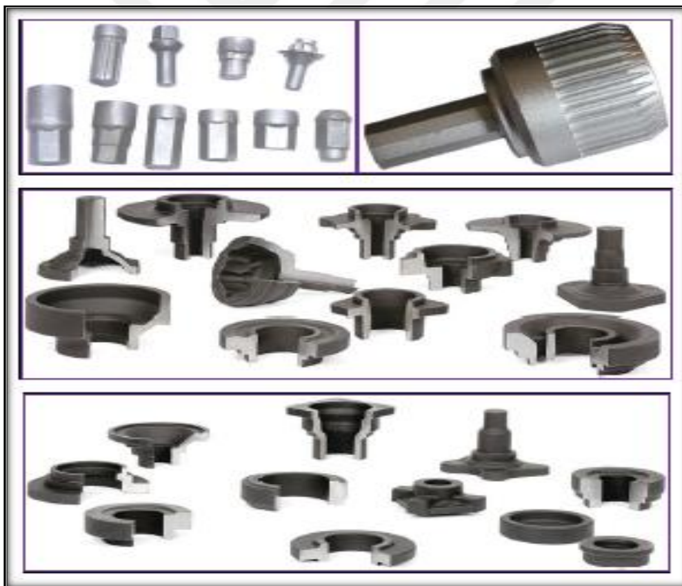
Figure 3.23: Applications of the combined extrusion process [4]
