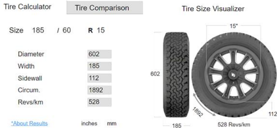
Figure 3.5. Wheel sizes of Toyota Yaris model vehicle (Adapted from [23].).
