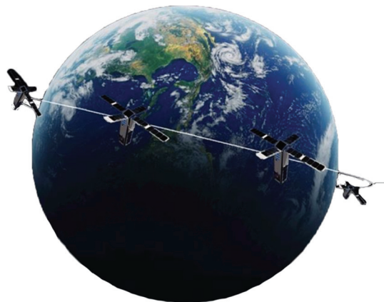
Fig. 4 CHESS 3U CubeSat constellation is a constellation of 3U CubeSats developed by the Swiss Federal Institute of Technology Lausanne. Its goal is to study high energy astrophysics with a hard X-ray
