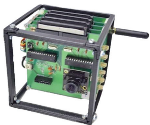
Fig. 6 KNACKSAT satellite, an acronym for KMUTNB Academic Challenge of Knowledge Satellite, is a 1U-CubeSat satellite (roughly 1.3 kg) developed by King Mongkut's University of Technology North Bangkok (KMUTNB), Thailand
