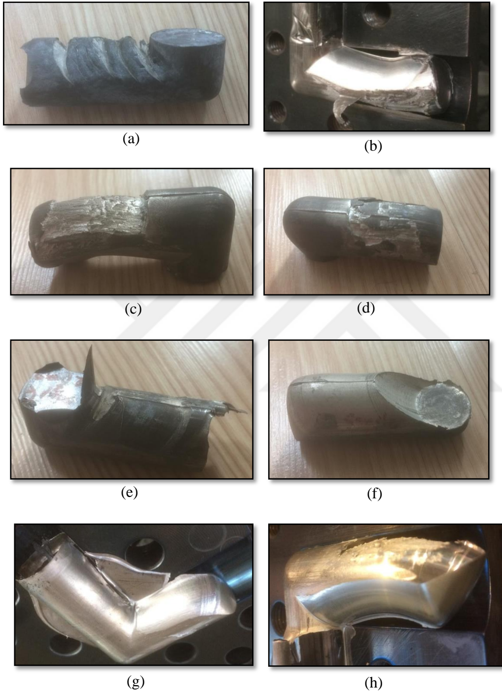
Figure 5.15: Product defects: (a) wrinkles; (b) flakes; (c) non-uniform shape; (d) cracks (e) flashes; (f) sloping ends (g) incomplete process; (h) curvature
