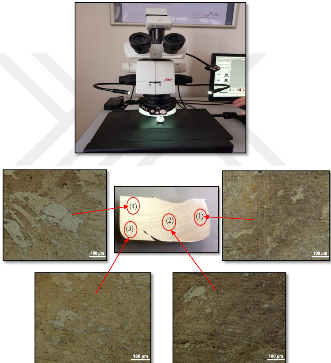
Figure 5.23: Microstructure of the sample
