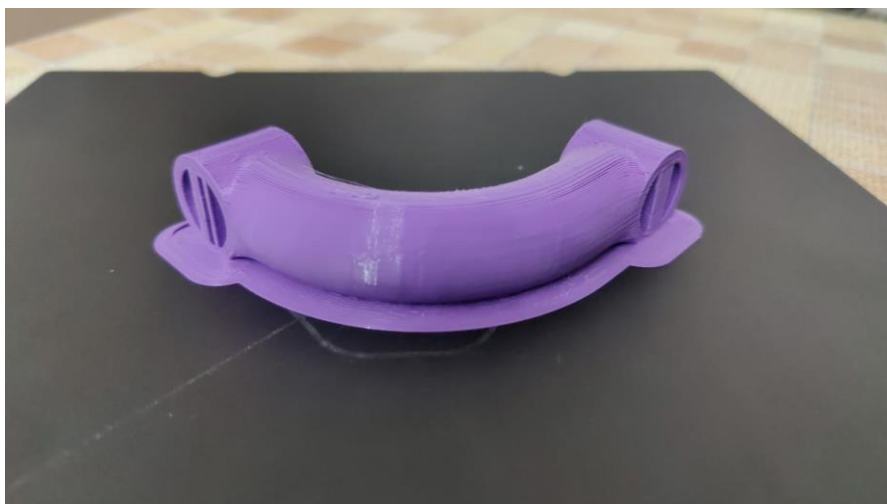
Figure 3. 20: 3D part with errors
