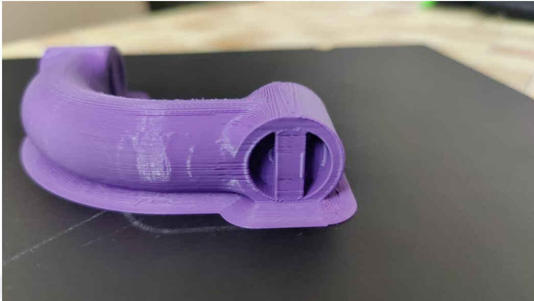
Figure 3. 21: 3D printed part with errors
