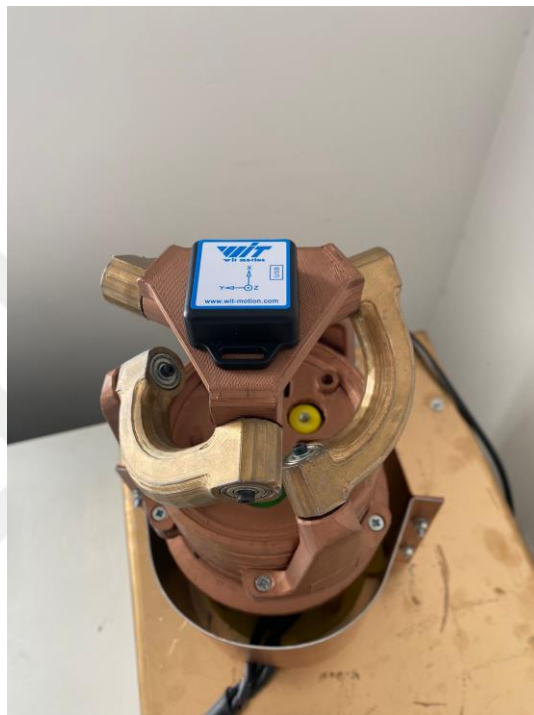
Figure 6. 2: SPM with BWT901CL IMU
