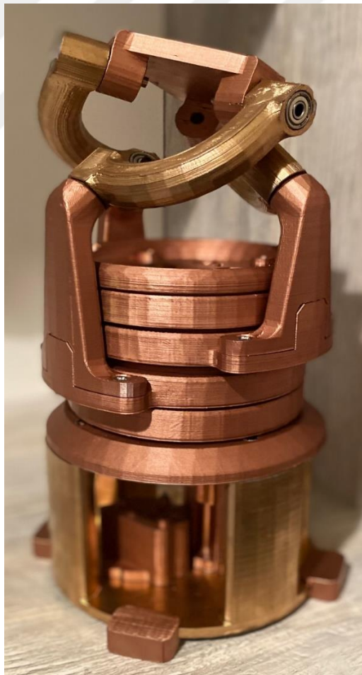
Figure 3. 1: Spherical Parallel Manipulator
