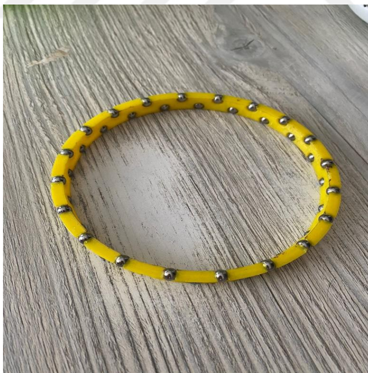
Figure 3. 12: Designed bearing for future work
