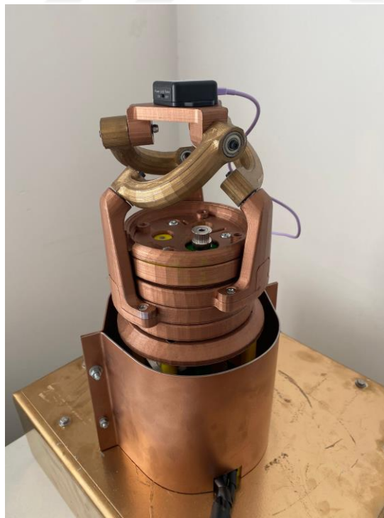
Figure 6. 1: SPM with IMU
